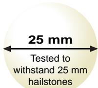
SolarPeak evacuated tubes are manufactured from high impact borosilicate glass (Like Pyrex), which is exceptionally strong. Evacuated tubes are designed to withstand 25 mm hailstones and temperatures lower than -50° Celsius.
